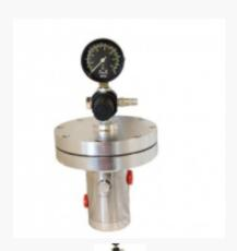
Use the fluid pressure regulator to reduce main line pressure, remove pulsations and to maintain the desired fluid pressure to the spray guns. Ecco Power Col has a compact design and high regulation accuracy. It introduces very little shear of the paint, is reliable and requires little maintenance. All wetted parts are made in stainless steel.
