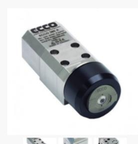
Ecco 380AA is an air assisted gun, designed to fit most types of high-pressure applications in automated production lines. Valve seat and needle tip are made in tungsten carbide for long durability. The gun can be changed in less than two minutes without any loss of mechanical precision or performance.
