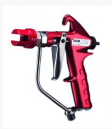
The manual spray gun Ecco 360 is a well tested gun, suitable for most high pressure applications. All parts in contact with the paint are made in stainless steel. The valve seat and the needle tip are made in tungsten carbide for long durability. The paint channels in stainless steel are designed as a protection guard in front of the trigger.
