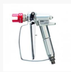
Ecco 510 is a multi-purpose manual high-pressure spray gun with exchangeable paint filter in the gun handle. The gun has an integrated swivel coupling for the paint hose connection, providing optimum freedom of movement when spraying in confined spaces. The 4-finger trigger makes the gun easy to operate also when using protection gloves. The EccoFlex airless hose is recommended for this gun.
