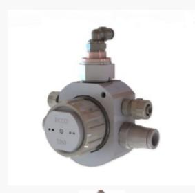
Ecco 81V is an automatic spray gun, especially designed for spraying objects inside confined areas. The control valve for opening/closing, as well as all connectors, are placed externally. The air cap is the only part that will be inside the spraying area during production.
