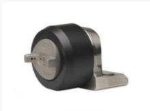
The automatic gun Ecco 71FA is especially suitable for spraying abrasive and wearing fluids like enamel. This gun has no paint needle and the material flow is controlled by an external valve. The gun is to be mounted on a mounting plate.
