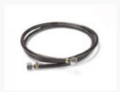
This EccoFlex paint hose is resistant to solvents, weak acids and to water at temperatures up to 100 °C. The outer layer is made of reinforced polyester and the inner hose is made of nylon. Order numbers below for standard length 8 metres, including coupling G 3/8 internal thread with cap nut.
