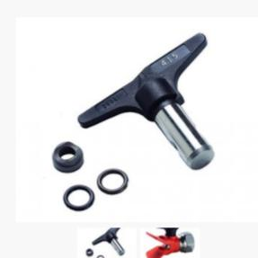
The Ecco Quick-tip can easily be cleaned by turning the tip 180° and a short paint blast will clear the spray tip orifice. The spray tip handle has an arrow, showing the spraying direction. The Ecco Quick-tip is manufactured from high quality tungsten carbide and stainless steel to ensure long lifetime in production. The holder for Ecco Quick-tip is available with thread that suits all airless spray guns.
