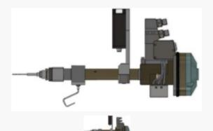
Ecco 480 is a new applicator complementing the Ecco 470 range specifically for cosmetic sealing. This 480 with dual nozzles was designed for roof ditch sealing with higher than normal demands for aesthetic results on new top level cars produced in Germany.
