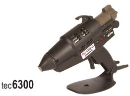
Extremely robust 43mm (13/4") spray glue gun with power-on light. Designed for industrial use, it sprays hotmelt at any angle with adjustable spray pattern. A non-toxic adhesive spray system, it covers large areas and applies hotmelt to heat sensitive substrates without damage. 8 bar (120psi) 85 l/min (3 cfm) air supply required.
