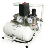
The tec-AIR 50TDC is an almost silent, compact, air compressor. It weighs just 21 kilos (46lbs), and comes complete with a robust tubular carrying frame. It is rated at 50 l/min (2.15cfm) and works to a maximum pressure of 8 bar (120psi). It is capable of operating up to two tec 6100 or tec 7100 applicators or one tec 6300 or tec 7300 spray applicator intermittently for small area coverage. It can also be used with most other pneumatic tools such as staplers, air brushes and tyre inflators.
